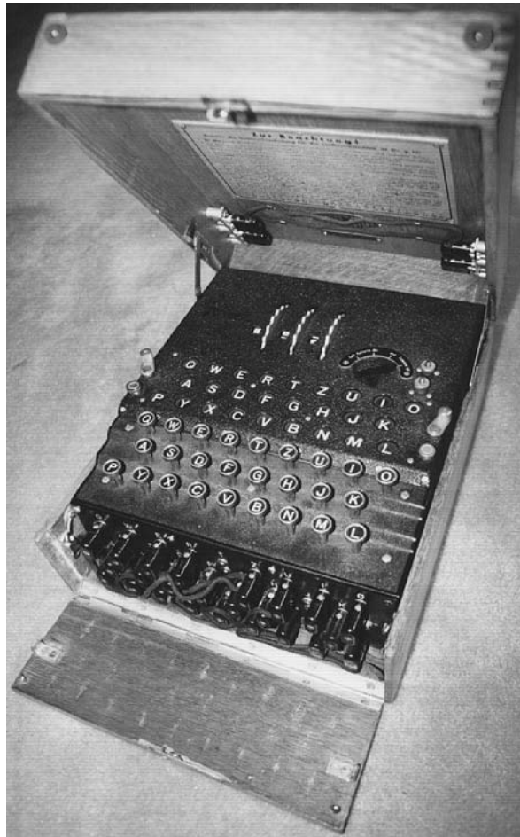
FIGURE 11.6 The Enigma machine. The machine has typewriter keys for entry, three rotors to define a letter substitution, a plugboard to implement a further substitution, and finally, lightbulbs to indicate the result.
