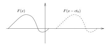
Figure 4. A traveling wave at two different moments in time: t = 0 and  $t = t_0$
