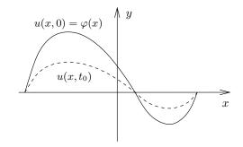
Figure 3. A standing wave at different moments in time: t = 0 and  $t = t_0$
