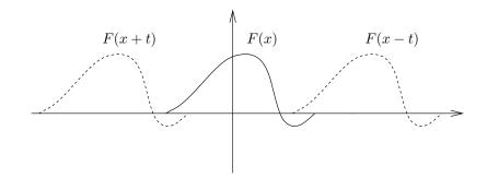
Figure 6. Waves traveling in both directions
