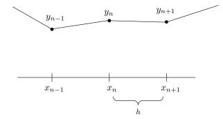
Figure 5. A vibrating string as a discrete system of masses
