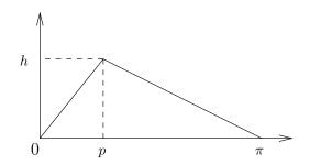
Figure 8. Initial position of a plucked string
