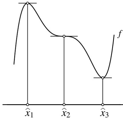
Figure 1.5 Illustrating the definition of stationary point.
