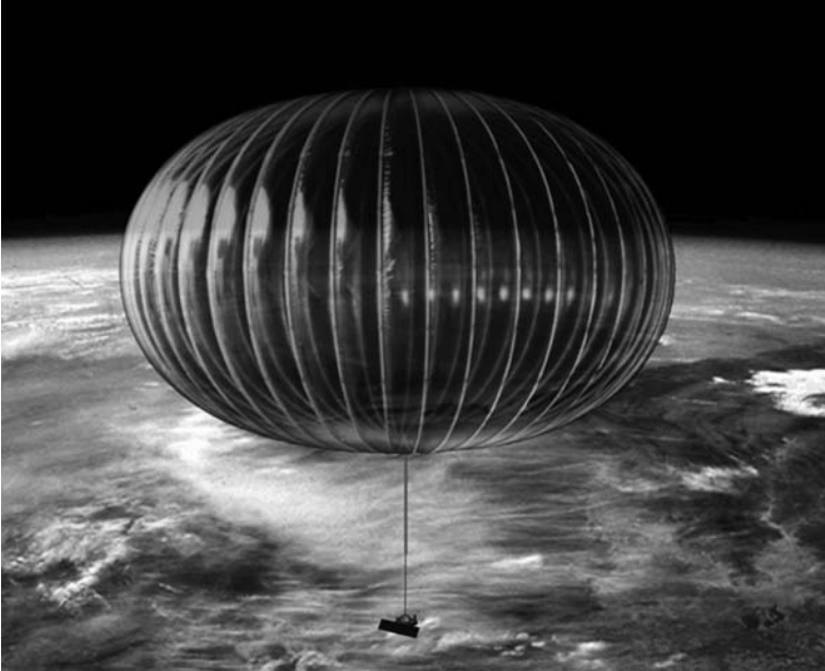
Figure 1.12 An artist's concept of NASA's Ultra Long Duration Balloon (ULDB), a structure composed of a lightweight polyethylene film about the thickness of ordinary plastic food wrap. Designed to lift 6000 pounds, it can rise to an altitude of about 33 km above 99% of Earth's atmosphere, for durations approaching 100 days. (Image courtesy of NASA)
