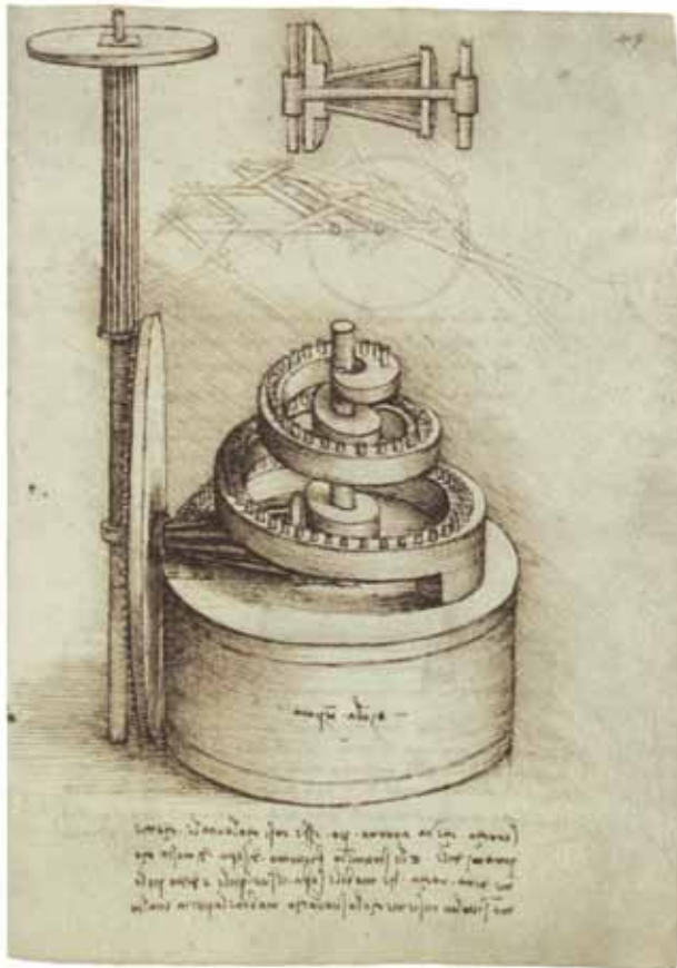
I-10. Leonardo, device for regulating springs. Madrid Codex I45r. Biblioteca Nacional, Madrid
