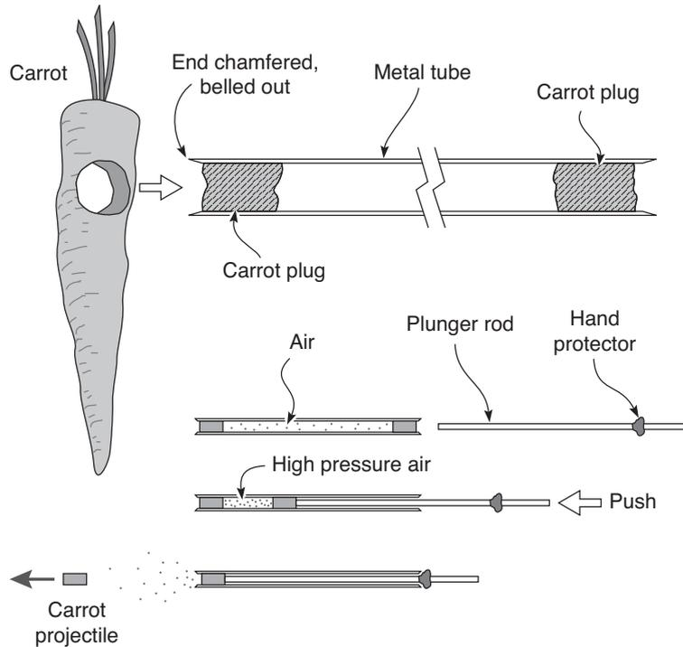
Now, if you are using copper tubing, it may help to widen both ends of the tube further by bellies the tubing out slightly as follows: insert the steel rod 1/2" to 1" into the tube and roll it around, so that it bellies out the ends of the tubing slightly. Copper tends to be surprisingly malleable and can be worked in this way quite easily. Repeat this process until you have a tube end 1 mm (1/32") or more wider than the body of the tube.
