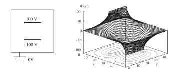
Figure 20.2 *Left:* A parallel-plate capacitor within a grounded box. A realistic capacitor would have the plates closer together in order to condense the field. *Right:* A visualization of the electric potential for this geometry. The contours projected onto the xy plane give the equipotential surfaces.
