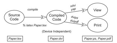
Figure 22.1 The steps followed and utilities used in preparing a document with LATEX. The source file is Paper.tex, the device-independent file is Paper.dvi, and the file ready for printing/posting is Paper.ps or Paper.pdf.
