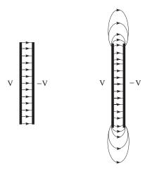
Figure 20.1 *Left*: Electric-field lines betweens the plates of an ideal parallel-plate capacitor. The equal spacing and single direction indicate a uniform field. *Right*: A representation of the field between the plates of a realistic capacitor. The field tends to "fringe" and extend beyond the ends of the plates.
