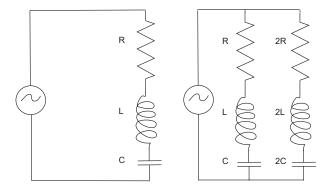
Figure 16.1 *Left:* An RLC circuit connected to an alternating voltage source. *Right:* Two RLC circuits connected in parallel to an alternating voltage. Observe that one of the parallel circuits has double the values of *R*, *L*, and *C* as does the other.
